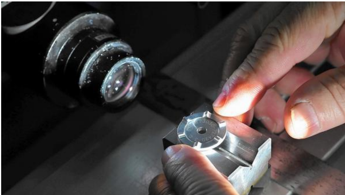
One of the Horst precision components, a spring seat for an aerospace application, is inspected on an Optical Comparator. (STEPHEN DUNN / Hartford Courant)
