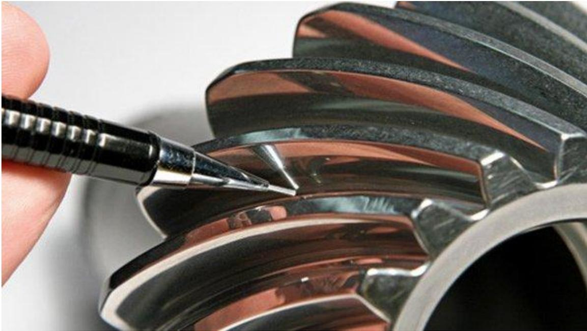
Superfinished spiral bevel gear teeth are seen on a component made by Aero Gear of Windsor. (Courtesy Aero Gear / June 25, 2012)
